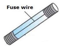
The wire inside the conductor melts and breaks the circuit as soon as the heating due to current increases.
