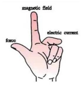
So, as mentioned magnetic force, magnetic field and electric current all are perpendicular to each other.
