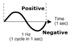
In the picture there is only one complete wave in a second, hence its frequency is 1 hertz. Which means that the coil has completed one revolution. Hence we can that <u>in</u> one revolution the current change its direction twice first positive than negative.
