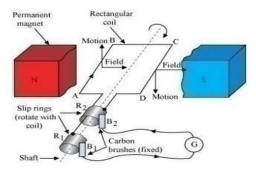
The parts of AC generator are:
