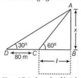
Here AB is the pole of height x metres and BC is one side of the square field of length l metres.
