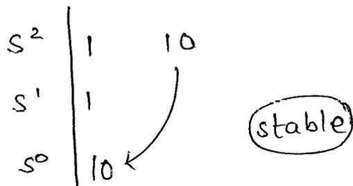
Q:- Find the range of k values to the given system for system stability.
