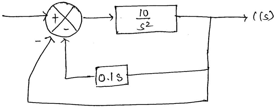
$$\Delta = 1 - \left[ \begin{array}{cc} -\frac{10}{s^2} & 0.1s \\ \frac{10}{s^2} & -1 \end{array} \right] = 0$$
