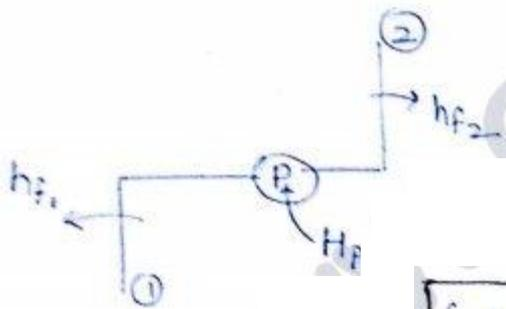
$$\left( \frac{P_1}{\rho} + \frac{V_1^2}{2g} + z_1 \right) - \left( \frac{P_2}{\rho} + \frac{V_2^2}{2g} + z_2 \right) = h_{f1} + h_{f2}$$
