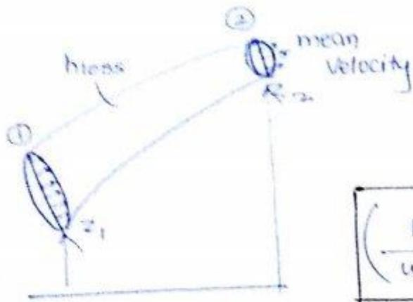
$$\left( \frac{P_1}{\rho} + \frac{V_1^2}{2g} + z_1 \right) - \left( \frac{P_2}{\rho} + \frac{V_2^2}{2g} + z_2 \right) = h_L$$
