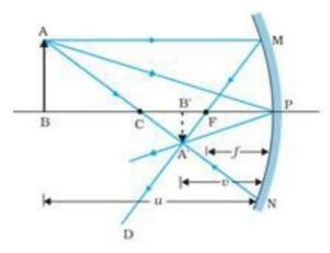
In  $\Delta A'B'F$  and MDF $\angle A'FB' = \angle MFD$  (Vertically opp. $\angle$ 's.)
