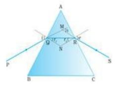
$\angle A + \angle Q + \angle O + \angle R = 360^{\circ}$
