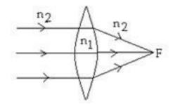
(2) When  $n_1 = n_2$  the lens behaves as a plane plate so no refraction takes place
