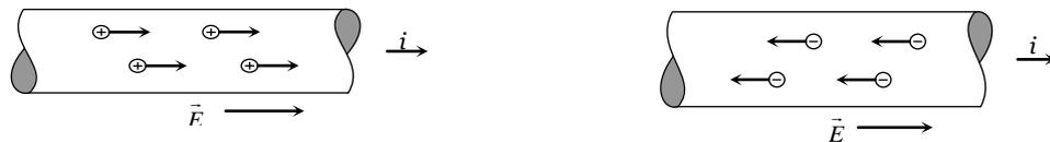
Though conventionally a direction is associated with current (Opposite to the motion of electron), it is not a vector. It is because the current can be added algebraically. Only scalar quantities can be added algebraically not the vector quantities.
