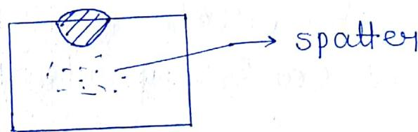
Due to excess amount of heat input liquid metal can be splash off to the base metal will form a rough surface know as weld spatter.
