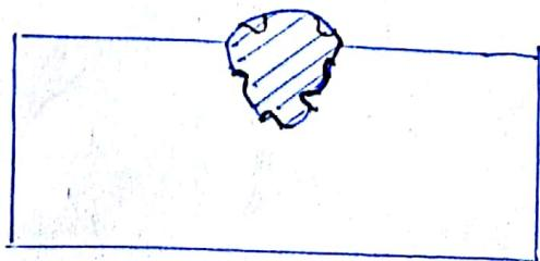
Due to ~~excess~~ lack of heat input and excess amount of welding speed filler metal is not fused properly with base metal and depth of penetration is less.
