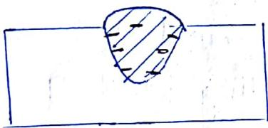
→ Due to non uniform cooling internal stress will be developed inside the weld weed.
