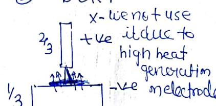
② Initial oxide layer present but due to e<sup>-</sup> movement from -ve to +ve so Oxide layer also move with e<sup>-</sup> Oxide layer can be remove by preceding inert gas this process called cathodic cleaning
