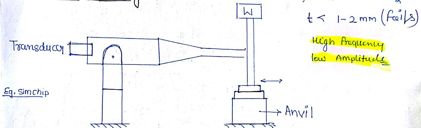
For joining of less thickness object like foils this technique can be used. Ultrasonic vibration are produced using transducer. They will be transfer to the workpiece through clamp. Due to vibration at the contact of two surface due to rubbing action heat will be generated. After reaching 30-40% to melting temp. by applying external load joint can be formed at the contact of two surfaces.
