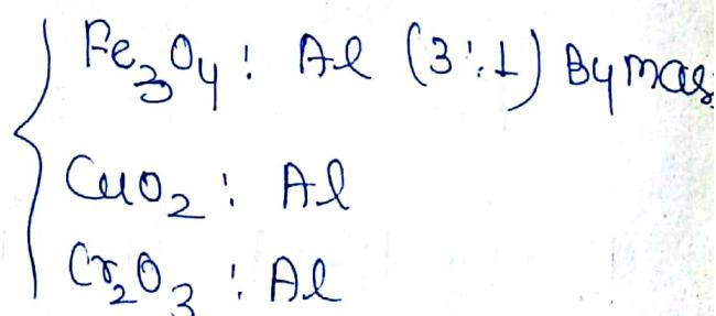
Thermite mixture can be heated in a crucible upto  $1200^{\circ}\text{C}$  by using 'Mg' rods. At this temp due to thermite reaction heat will be produced by using the heat iron will melt and it will be enter in workpiece. By allowing the liquid metal to solidify Joint can be produce,  $\text{Al}_2\text{O}_3$  will be acting as a slag.
