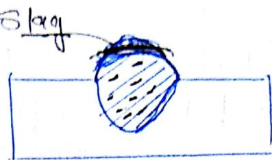
Due to lack of heat input and ~~insuff~~ improper positioning of welding torch with workpiece, if the slag is trapped inside liquid metal will form slag inclusion.
