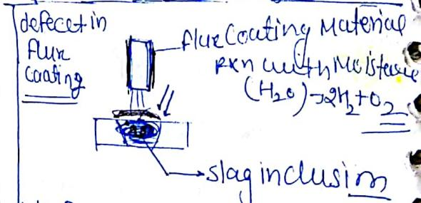
\* In Flux Coated we cannot do welding on Al, Mg, Alloy because it form  $Al_2O_3$  it will not allow metal to go inside.
