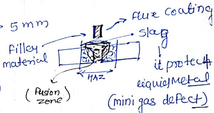
Welding:- It is a process in which localized permanent joint can be produced with or without application of heat, with or without application of pressure or pressure alone and with or without application of filler material for joining of similar or dissimilar materials.
