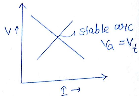
Problem:- Arc length voltage characteristic are given by  $V_a = 124 + 4 l_a$ ,  $V-I$  characteristic assumed as static line with open circuit voltage  $V_o = 80V$  & short circuit current  $I_s = 600A$  determine opt<sup>m</sup> arc length for max<sup>m</sup> power.
