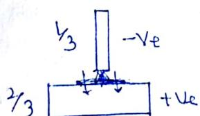
① possibility of oxide formation so we can't do Al, Mg, Alloy welding
