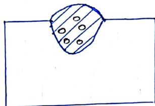
If the liquid metal is ~~too~~ absorbing gasses from atmosphere and they will trapped inside the weld bead will form gas porosity.
