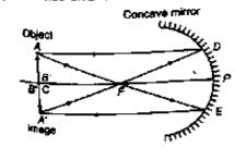
(v) When the object is between F and C. The image is formed beyond C and is inverted, real and larger than the object.
