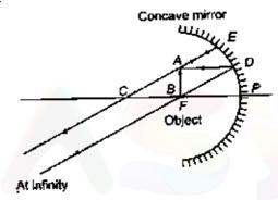
When the object is between F and P. The images formed behind the pole. The image is virtual, erect and large.
