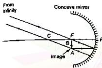
(ii) When the rays are parallel to the principal axis. The image is formed at F.
