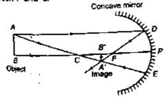
(iv) When the object is at C. The image formed is inverted, real, equal in size and is formed at C itself.
