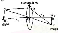
Object between f1 and 2f1. The image formed is beyond real inverted and magnified.
