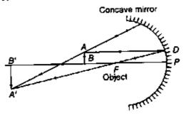
(vi) When the object is at focus. The image is formed at infinity. The image is real, inverted and infinitely large in size.
