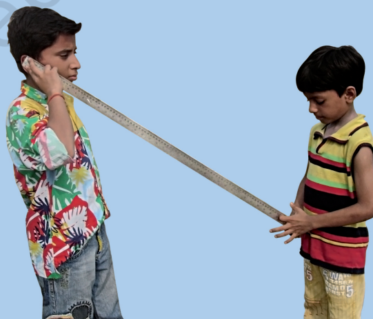
Fig. 13.12 : Sound travelling through a metre scale
