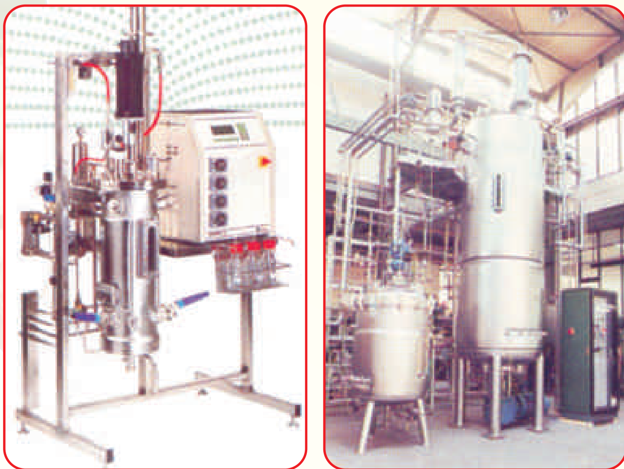
Fig. 4. (A) Laboratory-scale fermentor; (B) Industrial-scale fermentor.
