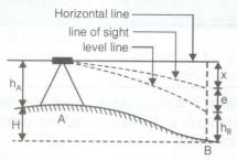
x = error due to inclined line of sight, and Here, e = error due to curvature and refraction
