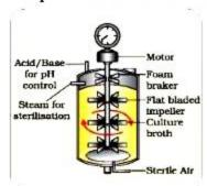
iii. The stirrer facilitates even mixing and oxygen availability throughout simple-stirred tank bioreactor, whereas in case of sparged stirred tank bioreactor, air is bubbled throughout the reactor for proper mixing.
