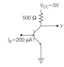
In the circuit shown, the value of  $\beta$  of the transistor is 48. If the supplied base current is 200 µA, what is the voltage at the terminal
