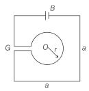
As shown in the figure, a single conducting wire is bent to form a loop in the form of a circle of radius r concentrically inside a square of side *a*, where  $a: r = 8: \pi$ . A battery B drives a current through the wire. If the battery *B* and the gap *G* are of negligible sizes, determine the strength of magnetic field at the common centre O.
