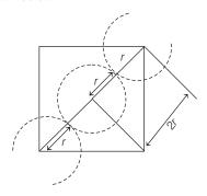
From the above figure, it is clear that the closest distance between two Au-atoms = 2r
