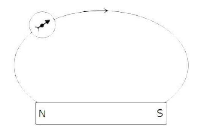
As the north pole of the magnetic needle is pointing in the opposite direction, so the nearer end of the magnet will be North Pole.
