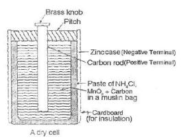
The strength of a fresh dry cell is 1.5 V. Cells of this kind which become useless once the chemicals inside them are used up are known as primary cells.
