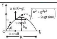
The horizontal component of velocity (u cosθ) remains constant where as the vertical component changes constantly due to acceleration due to gravity 'g'.]
