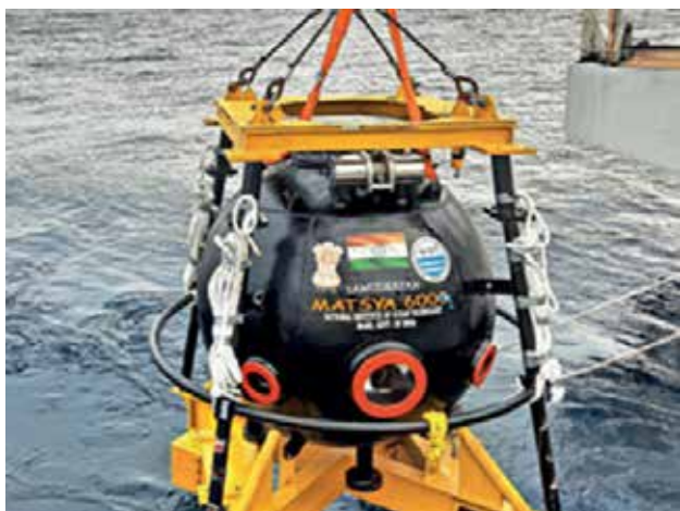
Marine reconnaissance submersible vehicle Samudrayan developed by the Ministry of Earth Sciences, Government of India
