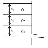
Assuming that the changes in  $h_1$ ,  $h_2$  and  $h_3$  are negligible, the instantaneous discharge velocity is:
