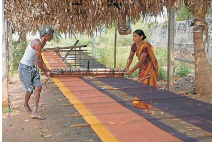
Fig. 7 Warp of sari being prepared.
