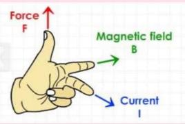
2 Right-hand Palm rule: Stretch the fingers and thumb of the right-hand at right angles to each other. To find the direction of the magnetic force on a positive moving charge, the thumb of the right hand ponts in the direction of velocity of particle v, the fingers in the direction of Magnetic Field B, then the Force F is directed perpendicular to the right hand palm
