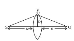
Thus a convergent lens is formed if  $\alpha = 2(n-1)D$ . This is independent of b and hence all paraxial rays from S will converge at O (i.e. for rays b << n and b << v).
