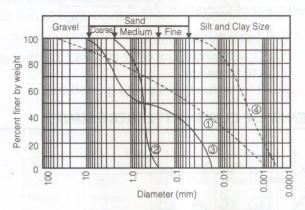
Curve-1: Well graded soil: good representation of grain sizes over a wide range and its gradation curve is smooth.
