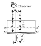
Now as a plane mirror forms image behind the mirror at the same distance as the object is in front of it, the distance of image I from mm' will be  $h + \left(\frac{d}{\mu}\right)$  and as the distance of virtual mirror from the front face of slab is  $\left(\frac{d}{\mu}\right)$ , the distance
