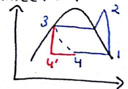
COP: In Ideal cycle  $\frac{RE}{W_{in}} = \frac{T_1 - T_4}{(T_2 - T_1) - (T_3 - T_4)} = \frac{1}{(r_p)^{\frac{\gamma-1}{\gamma}} - 1}$
