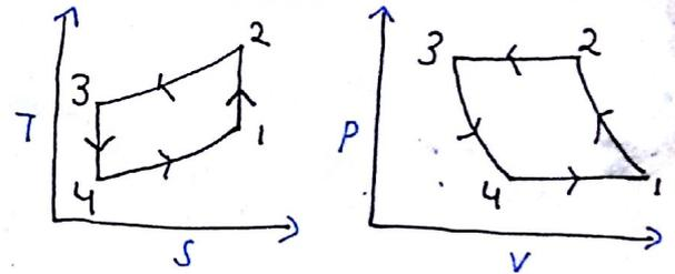
\* Here Expander not Throttle valve: As can't use  $h=c$  process b/c then  $T=c$  and with ↑ T heat absorption from storage not possible.
