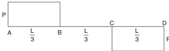
Figure shows shear force diagram of a beam  $ABCD$  of length  $L$ . Bending moment at the centre of the beam is
