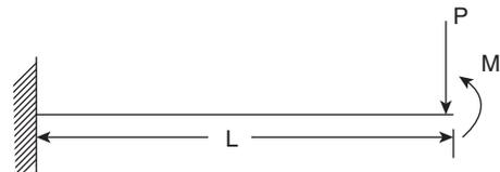
A cantilever beam of span  $L$  is subjected to a concentrated load  $P$  and a moment  $M$  as shown in the figure. Deflection at the free end is given by
