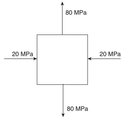
For the state of stress at a point in a stressed body, shown in figure radius of the Mohr's circle is
