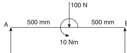
A simply supported beam of  $1 \text{ m}$  length is loaded at the mid span as shown in the figure. Maximum bending moment is
