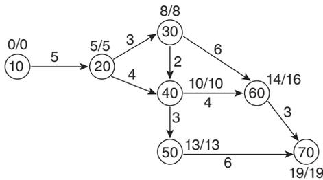
**Critical path:** 10 – 20 – 30 – 40 – 50 – 70 (or) Critical path is the path along which duration is maximum. From options, the path 10 – 20 – 30 – 40 – 50 – 70 has maximum duration. Choice (B)
