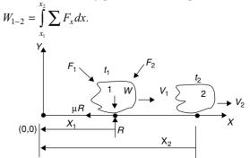
Change in kinetic energy from the positions 1 to 2 is  $(\Delta K \cdot E)_{1-2} = \frac{1}{2}m(v_2^2 - v_1^2)$
