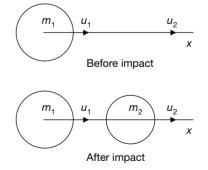
It is assumed that these velocities are directed along the line joining the centers of the two spheres and are considered to be positive if they are in the positive direction of the *x*-axis. This is called the case of direct central impact. Two equal and opposite forces, i.e., action and reaction, are produced at the point of contact during impact. In accordance with the law of conservation of momentum, such forces cannot change the momentum of the system of two balls and hence,
