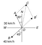
The vector  $\overline{OC}$  is the resultant velocity vector. Velocity of B is reversed and considered. Therefore the resultant is the velocity of A relative to B.
