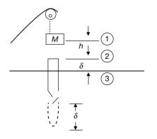
Given M = 800 kg, m = 400 kg, h = 1.2 m,  $\delta = 10 \text{ cm}$ .
