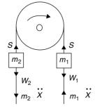
The inertia of the pulley and the friction on its axle are assumed to be negligible. If the motion of the system is assumed to be in the direction as shown by the arrow on the pulley, an upward acceleration  $\bar{x}$  of the weight  $W_2$  and
