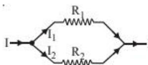
When such a combination of resistance is connected to a battery, all the resistances have the same potential difference across their ends.
