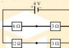
(i) current through  $6 \Omega$  resistor
