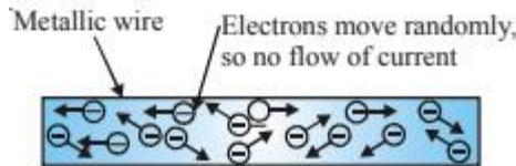
**Fig. Flow of electrons inside a metal wire when no potential is applied across its ends**
