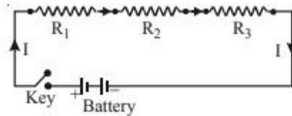
When a series combination of resistances is connected to a battery, the same current ( $I$ ) flows through each of them.
