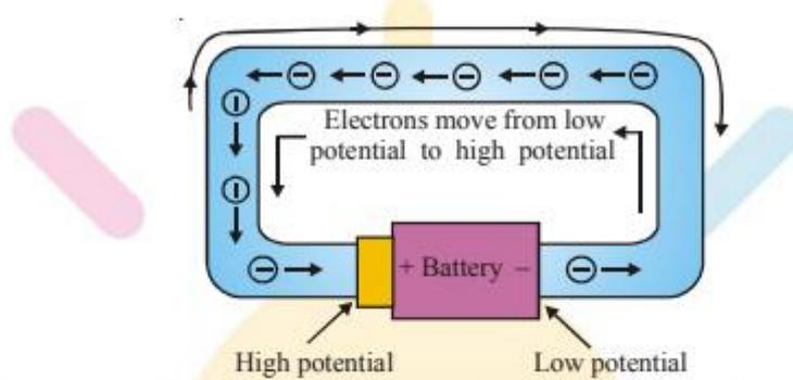
**Fig. Flow of electrons inside a metal wire when the two ends of a wire are connected to the two terminals of a battery**
