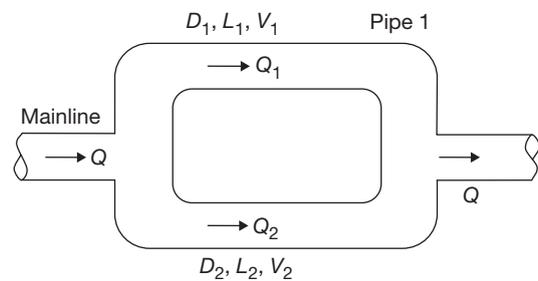
When pipes are arranged in parallel the head loss in each pipe is the same.
