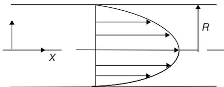
The average velocity of fluid in the pipe is
