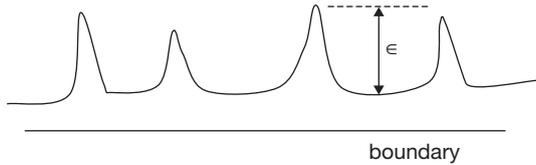
The variable  $\epsilon$ , referred to as *absolute roughness*, denotes the mean height of irregularities of the surface of a boundary. A boundary is generally said to be rough if the value of  $\epsilon$  is high and smooth if  $\epsilon$  is low. For a pipe, relative roughness =  $\frac{\epsilon}{D}$ , where  $D$  is the diameter of the pipe.
