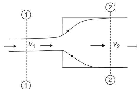
$$h_e = \frac{(V_1 - V_2)^2}{2g}$$
