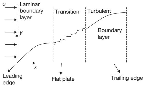
The above figure shows a boundary layer formed on a flat plate kept parallel to the flow of fluid of velocity  $u$ . Here  $u$  is called as the free stream velocity, sometimes denoted as  $u_\infty$ . The edge of the plate facing the direction of flow is called as the *leading edge* while its rear edge is called the *trailing edge*.
