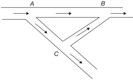
The pipe structure shown above can be converted into a pipe network (or hydraulic circuit) with nodes (or junctions) and links. Here  $Q$  denotes the flow rate and  $R$  denotes the flow resistance.
