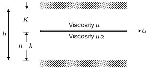
A large thin plate is pulled at a constant velocity  $U$  through a narrow gap of height  $h$ . On one side of the plate is filled with oil of viscosity  $\mu$  and the other side oil of viscosity  $\alpha\mu$ , where  $\alpha$  is a constant.
