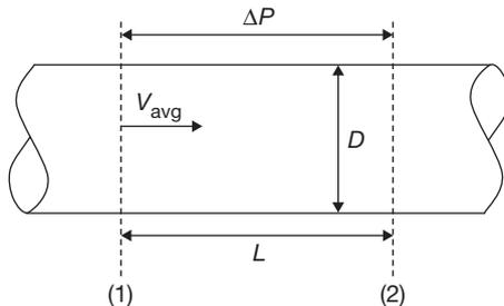
The pressure drop (between sections 1 and 2) across a length  $L$  of a flow section in a horizontal circular pipe of diameter  $D$ ,
