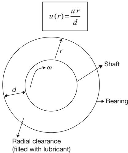
Where  $r$  is the radial distance from the outer surface of the shaft to the bearing,  $d$  is the radial clearance and  $u$  is the surface speed of the shaft. If the shaft is rotating at  $N$  rpm then,
