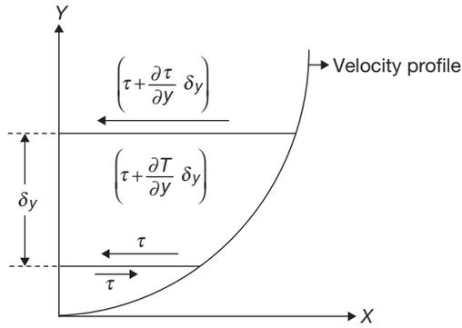
That is, the pressure gradient  $\left(\frac{\partial p}{\partial x}\right)$  in the direction of flow (steady and uniform) is equal to the shear gradient  $\left(\frac{\partial \tau}{\partial y}\right)$  in the direction normal to the direction of flow. The above equation holds for all flow conditions and geometries.
