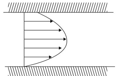
The discharge per unit width of the plates is given by,
