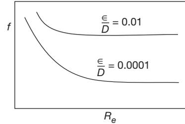
At very large Reynolds number,  $R_e$  friction factor curves in the Moody chart are nearly horizontal and thus the friction factor are independent of the Reynolds number.
