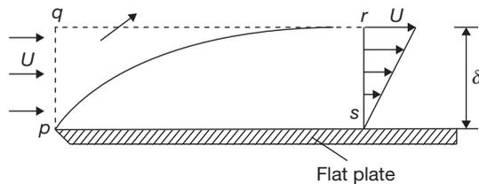
11. The mass flow rate (in kg/s) across the section  $q-r$  is:
