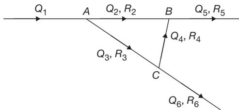
In the above network, the algebraic sum of the flow rates at any node must be zero, i.e., the total mass flow rate towards the junction must be equal to the total mass flow rate away from it.
