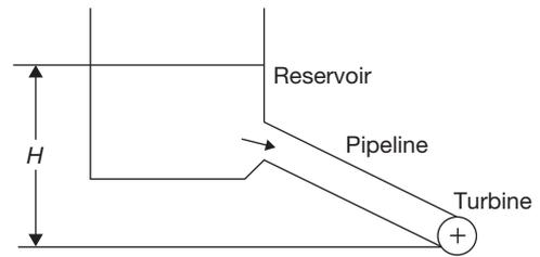
In the above system, hydraulic power is transmitted by a pipeline (through conveyance of the liquid) to a turbine. Here, the hydrostatic head of the liquid is transmitted by the pipeline.
