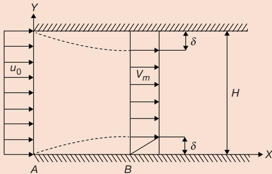
The velocity profile is uniform with a value of  $u_0$  at the inlet section A. The velocity profile at section B downstream is
