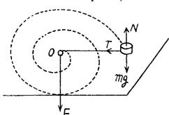
1.194 On the given system the weight of the body m is the only force whose moment is effective about the axis of pulley. Let us take the sense of  $\overrightarrow{\omega}$  of the pulley at an arbitrary instant as the positive sense of axis of rotation (z-axis)
