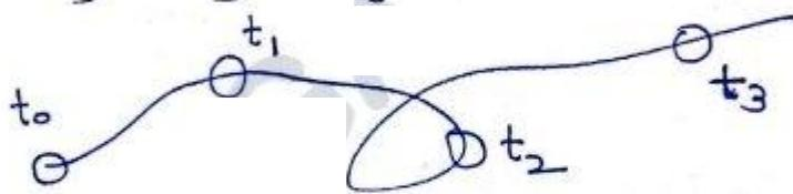
Streak line:— It is an instantaneous picture of all the particles passing through single point
