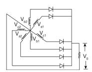
Two set of supply having a, b, c sequence 50 Hz and electrical Angle of 60° phase difference. Then the output signal frequency should be
