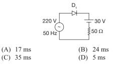
17. The circuit shown in figure produces an average output voltage of 59.30 V across the resistor. What will be the conduction Angle for SCR
