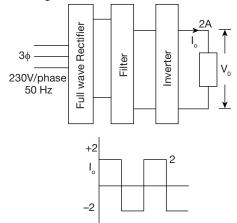
**32.** The output average voltage delivered by  $3\phi$  full wave rectifier of  $230 V_{phase}$ , 50 Hz in a converter inverter system of power supply will be
