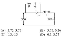
23. An SCR having turn on time of 5  $\mu$ s, latching current of 100 mA and holding current of 38 mA is triggered by a short duration pulse. What will be the minimum width, triggering pulse would require for successful turn ON of SCR
