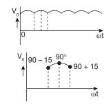
$$V_{\min} = V_m \sin(90 - 15) = 0.9659 V_m$$
