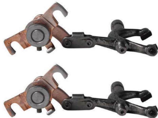
Figure 3.9.7 Gear selector mechanism
