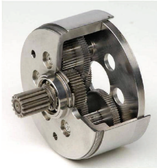
Figure 3.8 (b) Parts of overdrive
