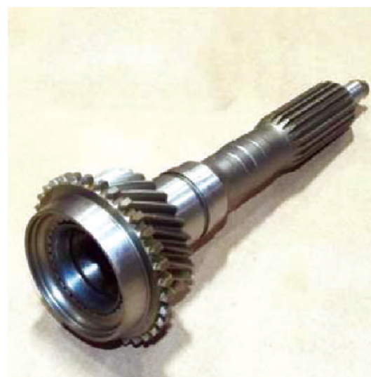
Figure 3.9.2. Gear box input shaft
