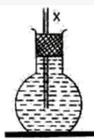
The level will rise above X when the flask is kept in hot water bath because the water in the flask will heat up and expand in volume thus raising the level of water in the tube above X
