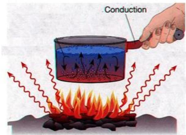
As shown in the picture, if the handle is made of metal/conducting substance, then heat will get transferred into your body & our hand will be burnt.
