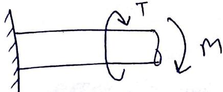
$$T_{max} = \frac{16}{\pi d^3} \left[ \sqrt{(K_b M)^2 + (K_t T)^2} \right]$$
