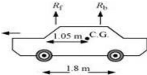
$R_f$  and  $R_b$  are the forces exerted by the level ground on the front and back wheels respectively.
