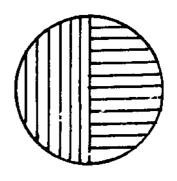
Therefore the amplitude transmitted in the present case will be  $\frac{A_1}{2\sqrt{2}}$  through either half.
