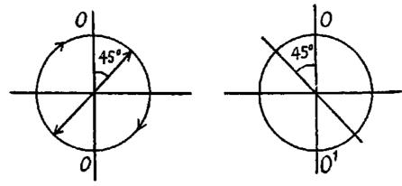
(b) If for any position of the plate the rotation of the polaroid (located behind the plate) does not bring about any variation in the intensity of the transmitted light, the incident light
