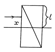
5.189 Light polarized along the x-direction (i.e. one whose electric vector has only an x component) and propagating along the z-direction can be decomposed into left and right circularly polarized light in accordance with the formula
