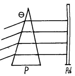
Let x = distance on the polaroid Pol as measured from a maximum. Then a ray that falls at this distance traverses an extra distance equal to
