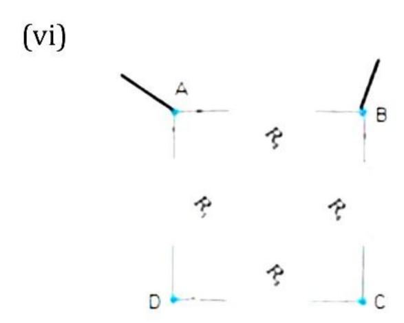
Resistances  $R_1 = R_2 = R_3 = R_4 = 2\Omega$  are connected, as shown in the diagram above. Between A and B, the series combination of resistors  $R_1$ ,  $R_3$  and  $R_4$  is connected in parallel with  $R_2$ . Total resistance between A and  $B = R_{AB}$ .
