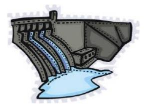
The barrage is equipped with sluices and turbines (similar to hydropower plants). Turbines generate electricity as the water flows out.
