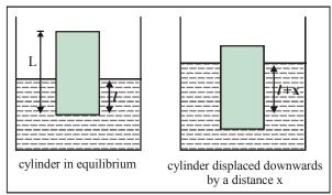
Mean position : cylinder is immersed upto  $\ell = \frac{Ld}{\rho}$
