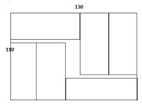
As seen from the fig. If following configuration is used max 6 number of tiles that can be accommodated on the floor.
