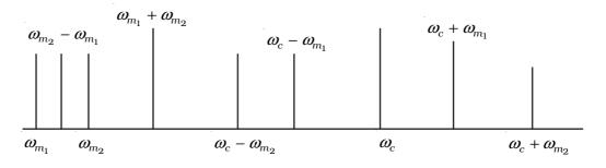
(ii) As can be seen frequency spectrum is not symmetrical about  $\omega_c$ . Crowding of spectrum is present  $\omega_c$ .
