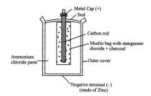
The chemicals in the cell react to produce current. A dry cell supplies current till the chemicals are exhausted and cannot react anymore.
