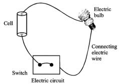
Electricity requires a path to flow from the positive terminal to the negative terminal of a cell. An arrangement or connection that provides the path to the current to flow from positive to the negative terminal outside the electrical cell via different electrical components is known as an electrical circuit.
