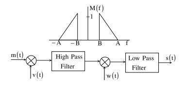
The bandwidth of the signal at the output of the modulator (in Hz) is \_\_\_\_\_. Answer: 60
