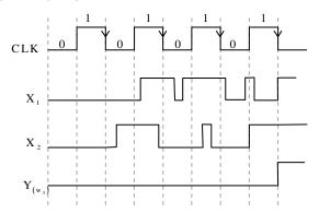
This is a synchronous circuit, so both the flip flops will trigger at the same time and will respond on falling edge of the Clock. So, the correct output (Y) waveform is associated to  $w_3$  waveform.
