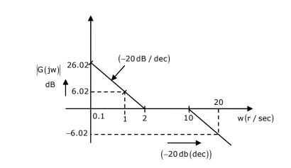
$\rightarrow$  Due to initial slope , it is a type-1 system, and it has non zero velocity error coefficient (K  $_v)$
