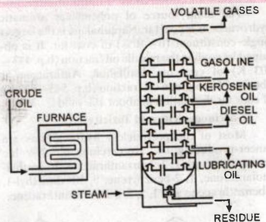
FIGURE 15.30. Fractional distillation of crude oil.
