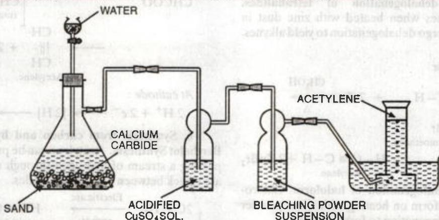
FIGURE 15.18. Laboratory preparation of acetylene.
