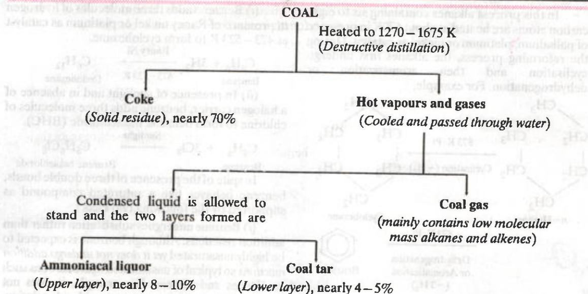
**FIGURE 15.20.** Flow chart of destructive distillation of coal.
