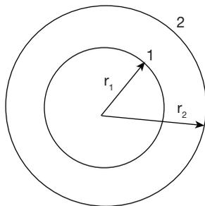
A solid sphere of radius  $r_1 = 15\text{ mm}$  is placed concentrically inside a hollow sphere 2 of radius  $r_2 = 75\text{ mm}$  as
