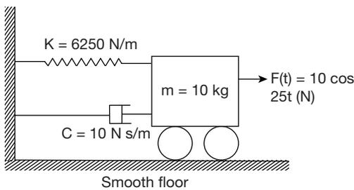
For the spring-mass-dashpot system shown in figure, the mass  $m = 10$  kg, stiffness of spring  $k = 6250$  N/m and damping coefficient of damper,  $C = 10$  N s/m. It is subjected to a harmonic force  $F(t) = 10 \cos 25t$  (N). The amplitude of forced vibration in the steady state, expressed in millimeter, is \_\_\_\_\_.
