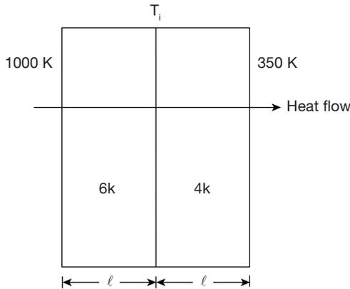
Heat transfer through a composite wall of two sections, each having same thickness ( $\ell$ ), is shown in figure. The thermal conductivity of one section is  $6k$  and that of the other is  $4k$  respectively. The left face of wall is at  $1000\text{ K}$  and right face at  $350\text{ K}$ . The temperature  $T_i$  (in  $\text{K}$ ) of the interface of the composite wall is .
