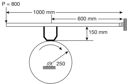
A drum brake of 250 mm radius is rotating in the clockwise direction as shown in the figure. The coefficient of friction between drum and shoe is 0.25. The braking torque (in N m) on the brake drum when an effort  $P = 800$  N is applied at the end of lever is .
