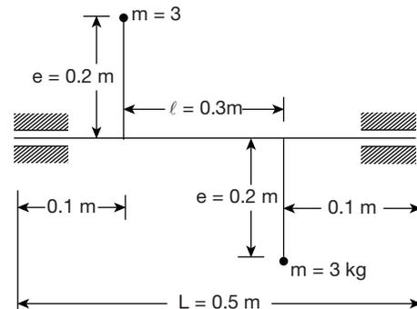
A strictly balanced system is shown in figure. Two equal masses, each equal to  $3\text{ kg}$ , each with an eccentricity  $e = 0.2\text{ m}$ , are placed on opposite sides of the axis in the same axial plane. The shaft rotates now at a constant angular speed  $\omega = 10\text{ rad/s}$ . The dynamic reaction at each support (in  $\text{N}$ ) will be .
