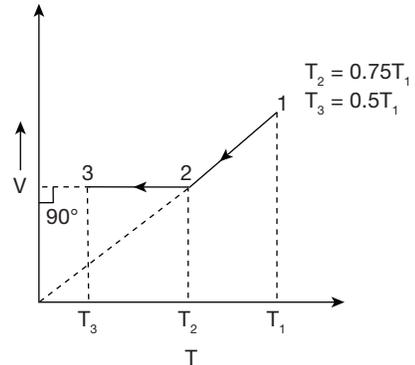
The ratio of final pressure  $p_3$  to initial pressure  $p_1$  of the gas (ie  $\frac{p_3}{p_1}$ ) is
