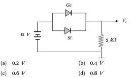
**27.** In the circuit shown in figure the maximum output voltage V is
