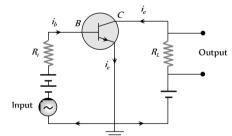
This has been shown a  $NP\overline{N}$  transistor. Therefore base emitter are forward, biased and input signal is connected between base and emitter.
