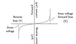
When the reverse voltage across the zener diode is equal to or 23. (a) more than the breakdown voltage, the reverse current increases sharply.
