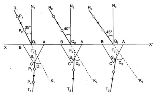
Fig. Refraction through prism at different angles.
