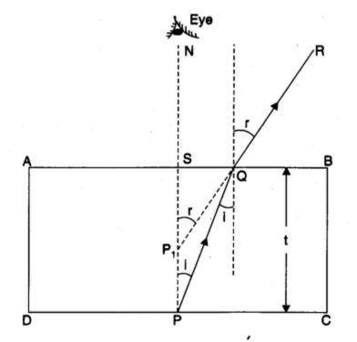
Fig. 9.06. Real and apparent thickness of a glass slab.
