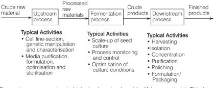
The upstream processing in biotechnology involves identifying a material. This forms the initial process of fermentation. It deals with inoculum preparation, preparation of culture media, scale up of the entire process and inoculation.
