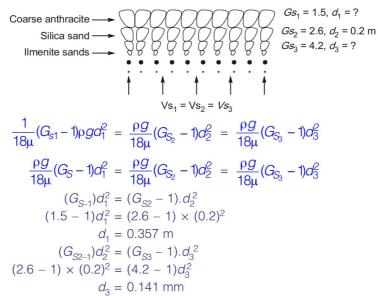
The logic is that if we are creating 3 layers for better filtration and if we want those layers to be intact, even after backwashing, then we need to ensure that as the backwashing is stopped, each layer settles with the same velocity so that the stratification is maintained as it is.
