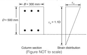
The maximum compressive strain ( $\varepsilon_c$ ) at highly compressive extreme fiber in concrete, where there is no tension in the section, is \_\_\_\_\_ × 10<sup>-3</sup> (rounded off to 2 decimal places).
