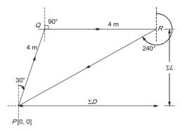
Horizontal distance of traverse from P to  $R = \Sigma D$
